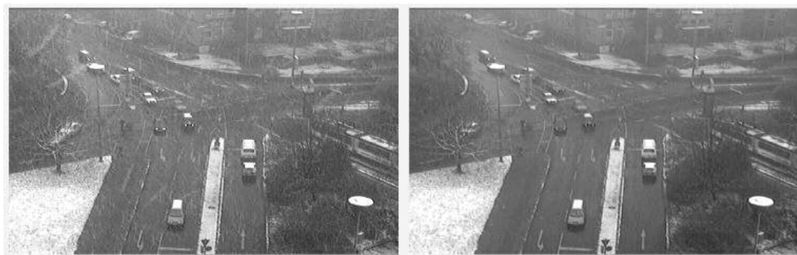
Fig.2 (Video frame on left showing a traffic scene while snowing. Note the streaks in the image due to the snow flakes. The same video frame after spatial and temporal smoothing is on the right, without the snow streaks) [22] .
